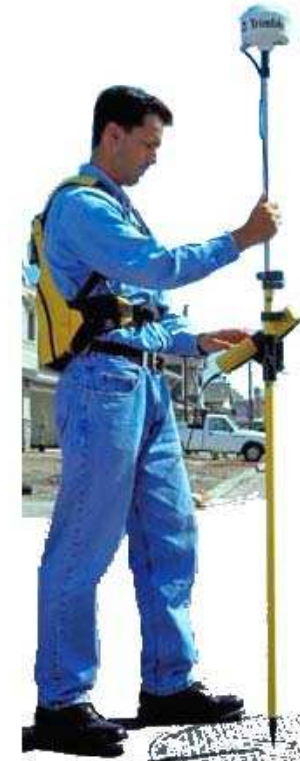
Rover unit: on a detail pole with power supply) to base station logger, power supply and receiver.
