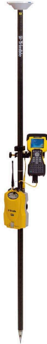
The data-logger gives current information on the condition of the constellation as well as the coding options needed to select points for mapping.
