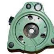
Tribrach, the base station can be re-occupied by an EDM or prism target if required: the standard traversing tribrach allows re-occupation with out re-levelling etc.
