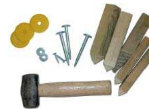
Station markers and detail pegs; if a feature needs to be pegged out for chain and offset survey from GPS tie points.
