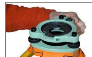
Fig 3.7.2 Right: from top: 1- The tribrach foot-screws are used 2 and 1 by turning the 2 screws 'thumbs out' or 'thumbs in' - never both thumbs in the same direction! 2- Levelling with the leg adjustment. 3- grip the tripod leg as shown and slide each leg in turn up or down as required to level the bubble. 4, 5- Bring the plummet back over the mark with the foot screws.
