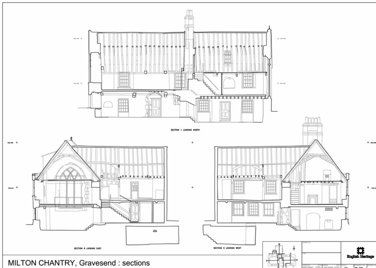
Fig 2.12 Sectional elevations laid out on a sheet with correct rubric: showing key plan, north point, authorship scale etc.
