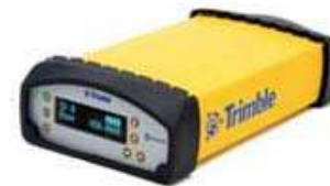
Base station radio relay unit: for DGPS this is essential, the unit relays the base station position to the rover to form the base line for the trilateration of each measured point.
