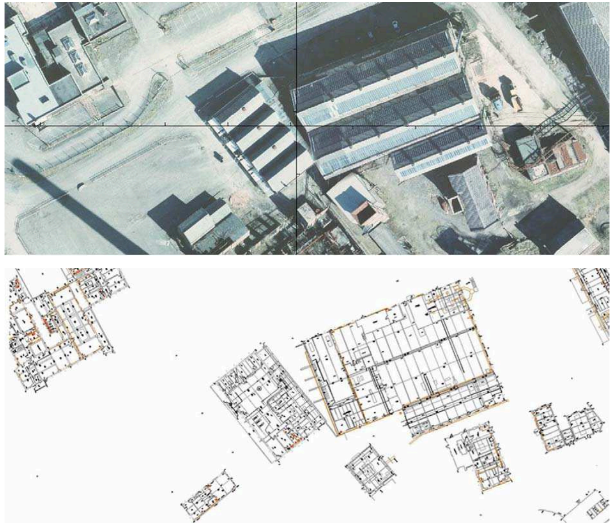
Fig 1.3 Undifferentiated and differentiated data. The orthophotograph (top) shows the power of undifferentiated capture by an indirect method: aerial photography which has rapidly revealed the nature of the site including, building types, roof configurations, land use, how the buildings are linked, their materials and condition. The measured plan of the buildings (bottom) tells a different story, resolvable to large scale (1:50) the building plans show the internal spaces, wall thicknesses and openings that will inform the re-use planned for consolidating the site. The differentiation in the building plans is the information has been SELECTED at capture for the purpose of building conservation.
