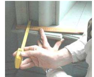
Surveyors rod (folding rule) being used as a chain line with offsets to moulding detail being taken by tape.
