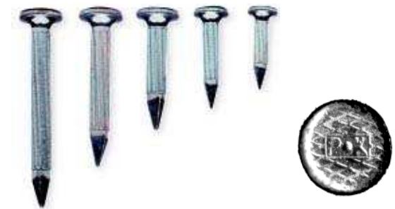
Fig 3.11 Station Markers: a selection of marks is usually needed. Parker-Kalon (PK) masonry nails are good for marks in masonry or tarmac. A clear centre mark is essential.
