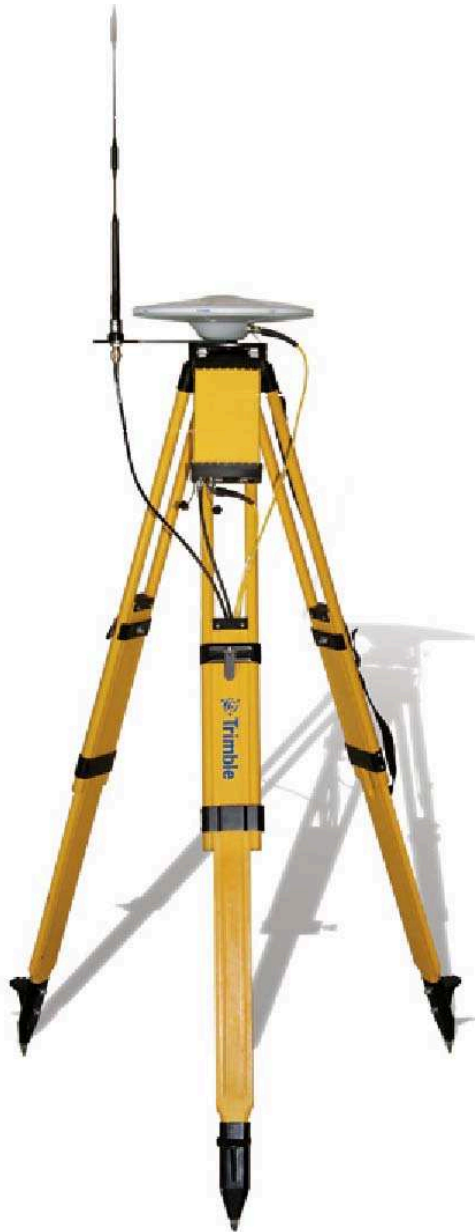
Base station receiver mounted on levelled tripod with repeater radio, antenna, and power supply.
