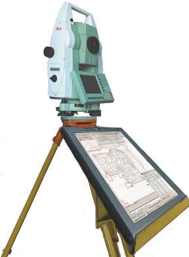
Fig 3.6 SEEING THE PLOTTED WORK AS IT'S MEASURED
