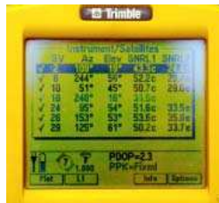
The data-logger gives current information on the condition of the constellation as well as the coding options needed to select points for mapping.
