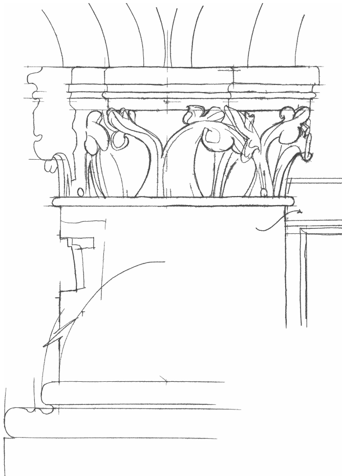
Fig 2.4: Sketch Diagram of a capital of the nave arcade, Inglesham, Gloucestershire. The survey required a CAD drawing for a sectional elevation. Due to multiple surface reflectance the REDM trace failed to delineate the details. The drawing clarifies the data.
