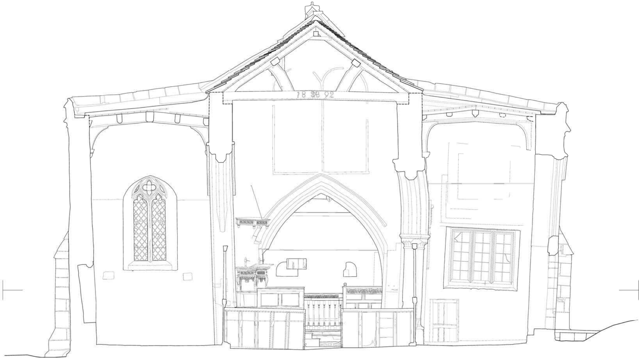
Fig 3.21 The cross section looking East. The section reveals the deformation of the nave arcade and the extent of the wall rotation on the south aisle. Small areas of incomplete detail in the roof voids and at wall plate height were the result of restricted access. The integration of measured drawing, digitised rectified photography and REDM has generated the completeness required for the sectional elevation.
